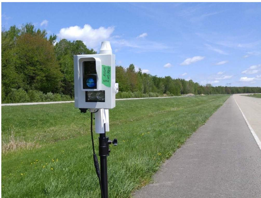
2. View of speed enforcement camera DFD-0 – SAFEPLACE ENFORCER CAM 24°.
