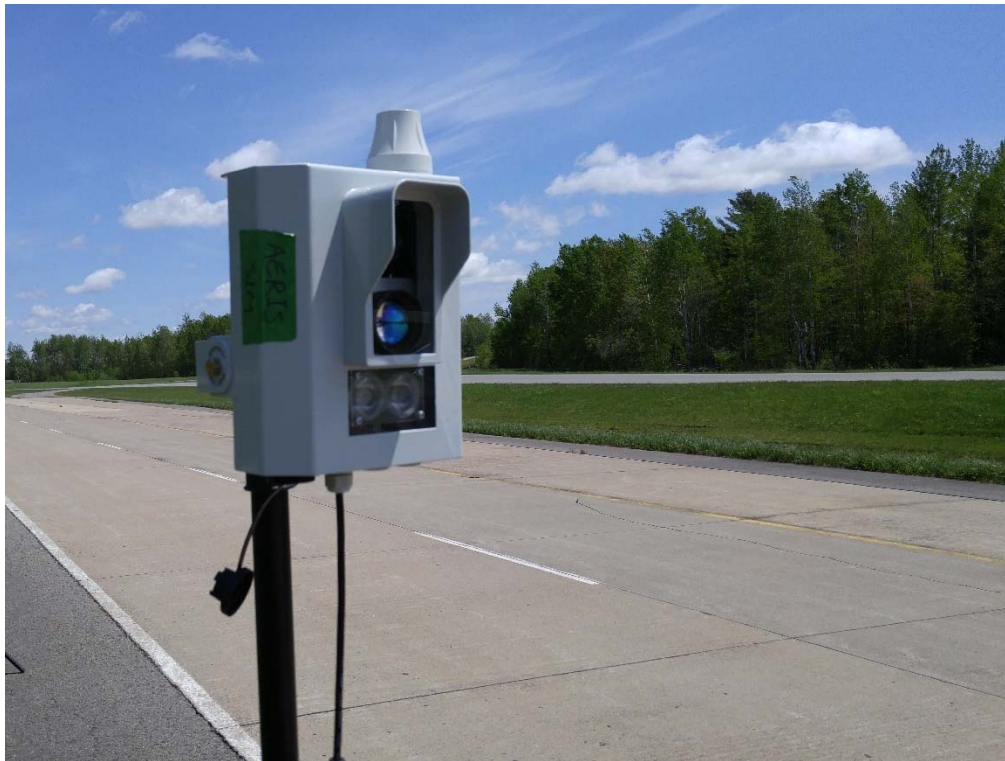
1. View of speed enforcement camera DFD-1 – SP ENFORCER CAM 18°.
