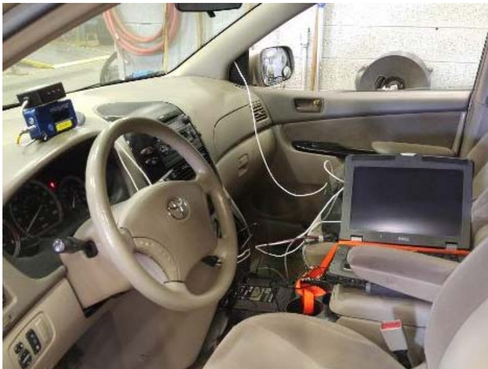
6. View of the instrumentation onboard the vehicle used for testing.
